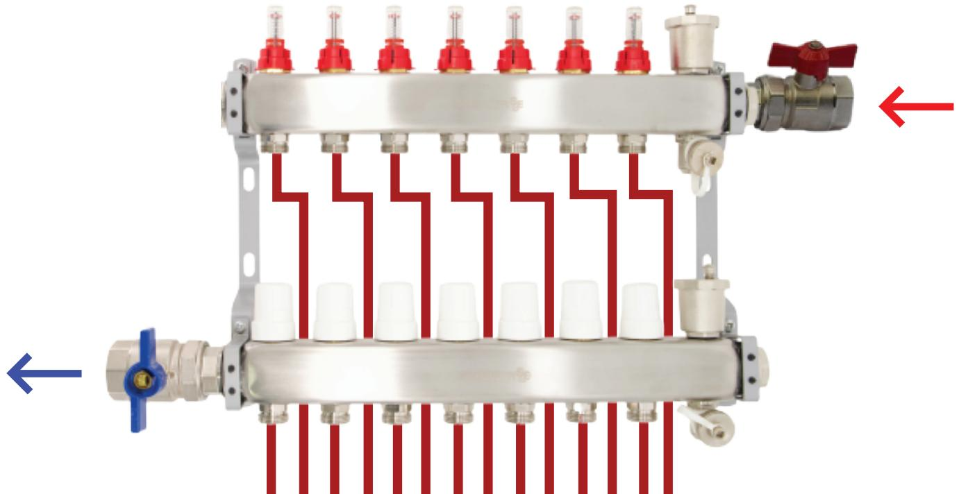
The Schuller manifold has an ambidextrous cap, meaning supply/return lines can be fed from either direction. It is recommended for installers to install one line on each end, to insure proper balancing in the manifold.
